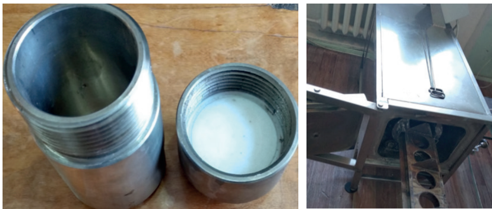
Figure 1 – Thermostatically controlled unit with autoclaves
